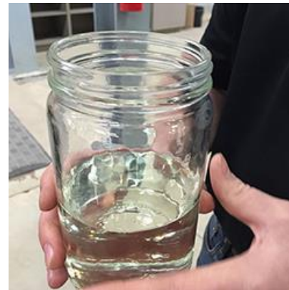
Example of Super™ biodiesel distilled at the final stage
