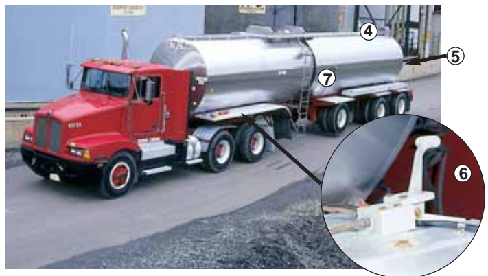
Top: Document Verification Middle: Typical Tank Truck Fittings Bottom: Tank Truck with Emergency Shutoff Valve (inset)
